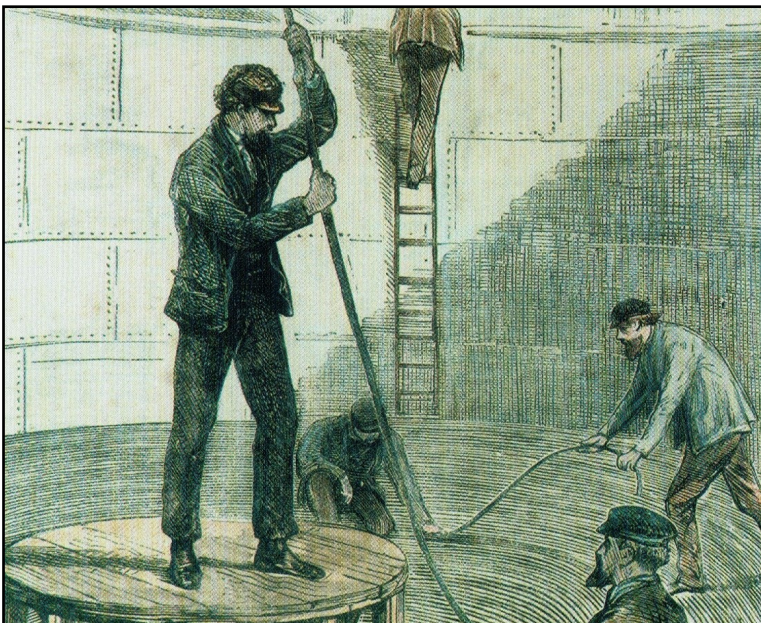
Coiling down the cable in the tank
